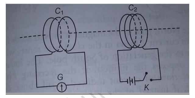
The galvanometer shows a momentary deflection when the tapping key K is pressed. The pointer in the galvanometer returns to zero immediately. If the key is held pressed continuously, there is no deflection in the galvanometer. When the key is released, a momentary deflection is observed again, but in the opposite direction. It is also observed that the deflection increases dramatically when an iron rod is inserted into the coils along their axis.
