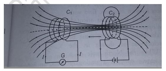
If the bar magnet is replaced by a second coil  $C_2$  (as shown in figure given above) connected to a battery. The steady current in the coil  $C_2$  produces a steady magnetic field. If coil  $C_2$  is moved towards the coil  $C_1$ , then the galvanometer shows a deflection. This indicates that electric current is induced in coil  $C_1$ .
