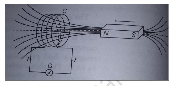
If North-pole of a bar magnet is pushed towards the coil, the pointer in the galvanometer deflects, indicating the presence of electric current in the coil. This deflection lasts as long as the bar magnet remains in motion.
